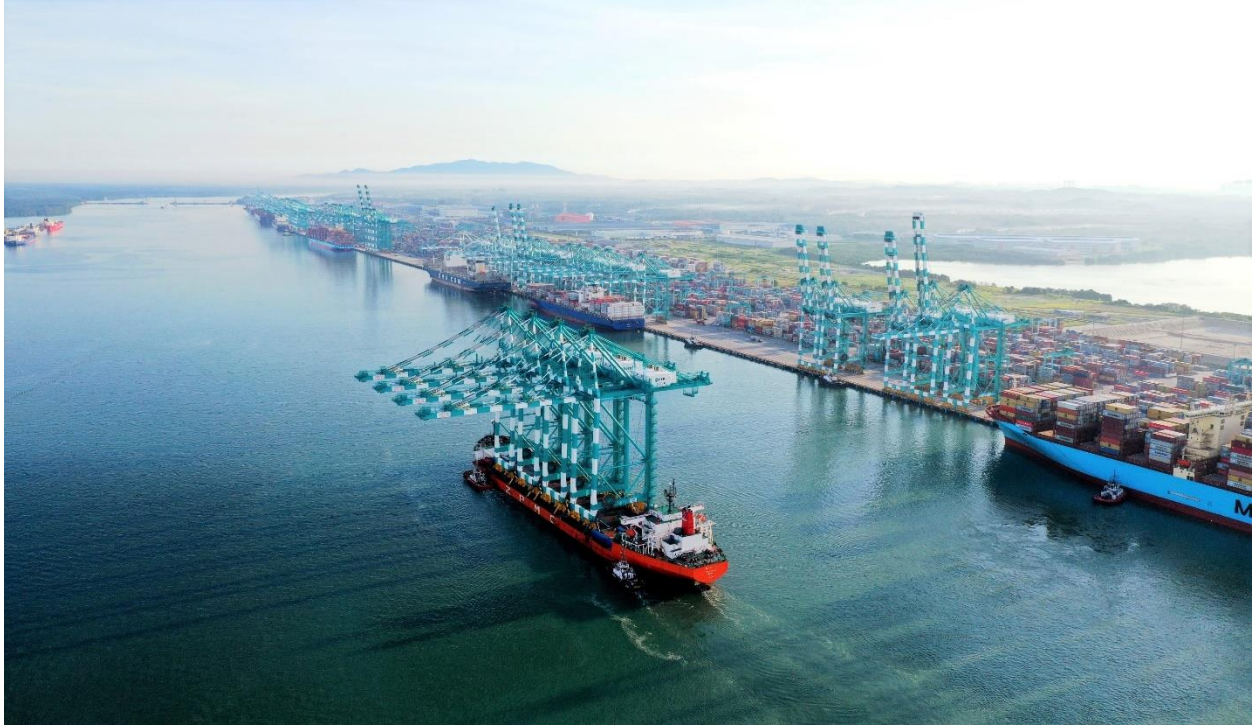
Photo Caption: The arrival of 4 new ship to shore (STS) quay cranes at PTP
